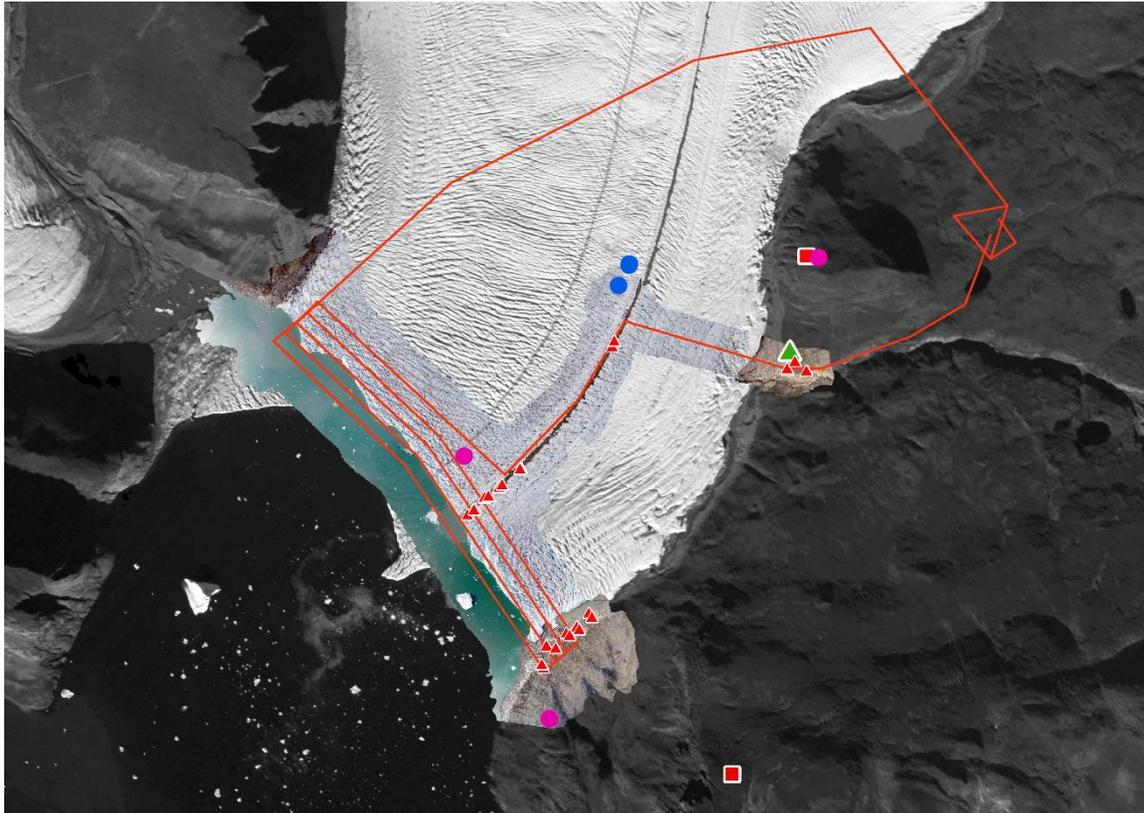
*Figure 2: Flight plan (red line) of the calving front monitoring and the DGPS measured Ground Control Points (red triangles).*
